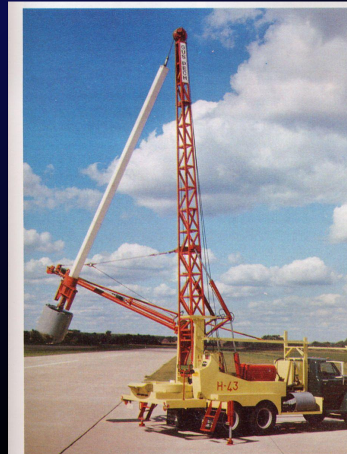
Figure 10.47. Bucket auger rigs can be used to construct water wells in weakly consolidated formations. (Gus Pech Manufacturing Co., Inc.)
